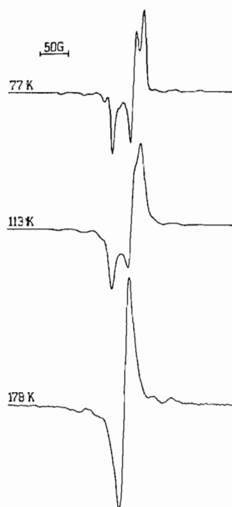
Fig. 8. X-band ESR spectra of 2.5 mM \alpha_1 I in acetonitrile recorded at 77, 113 (isopentane/liquid nitrogen) and 178 (toluene/liquid nitrogen) K.
